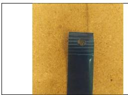
Mechanically Punched Hole – Prior to Testing
