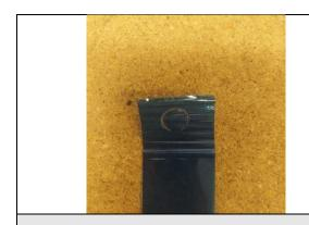
Hot Punched Hole – Prior to Testing
