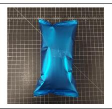
Sealed Package – 0.25-inch Width of Seal
