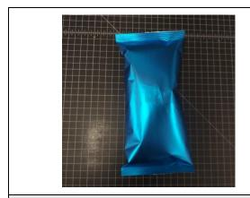
Sealed Package – 0.5-inch Width of Seal
