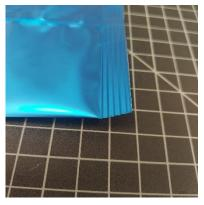
Package Seal – 0.5-inch Width of Seal
